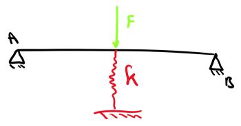
Determine the value of k needed to reduce the deflection of the beam by 25 percent of its original value.
