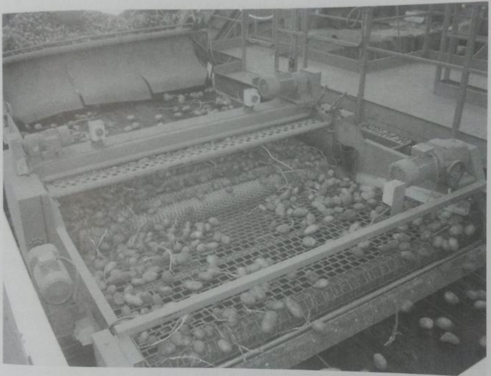
Fig. 11.4. Star wheel dry cleaner followed by endless screen grader. (Courtesy of RJ Herbert Engineering Ltd, Cambridgeshire, UK.)
